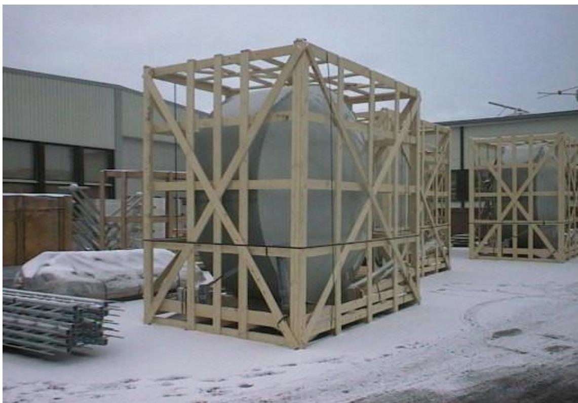
By default, Aerial Oy radio relay antennas are shipped in palette based wooden crates.
